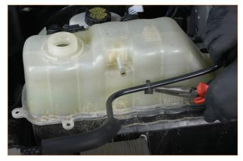
Disconnect the vacuum supply hose from the vacuum manifold attached to the rear of the primary degas tank. (1x quick-disconnect fitting).
