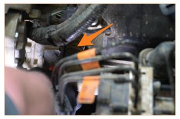
**16.** Mark the battery tray as shown in the image below. This is where the battery tray must be cut to remove the stock degas tank.
