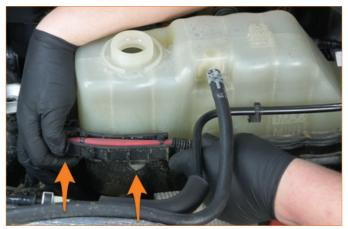
08. Remove the upper hose from the primary degas tank. (1x spring clamp).
