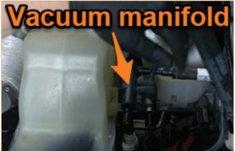
Disconnect the lower hose from the primary degas tank. (1x spring clip).
