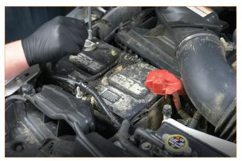
**04.** Remove the battery tie down from the primary battery and then remove the battery from the vehicle. (2x 10mm nuts).
