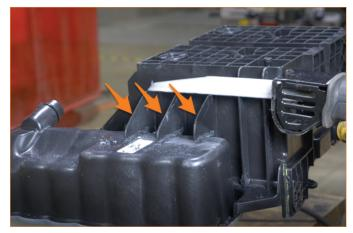
19. Using the cut made in step 17 as a guide for the cutting blade, use a reciprocating saw to finish removing the stock degas tank from the battery tray.
