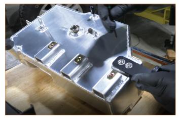
Attach the MM2356-03 bracket and MM2356-01 degas tank to the battery tray using the 3x long 5mm allen bolts. Leave the bolts loose. (3x long 5mm allen bolts).
