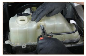
**09.** Remove the vacuum supply hose retainer from the primary degas tank. (1x clip).
