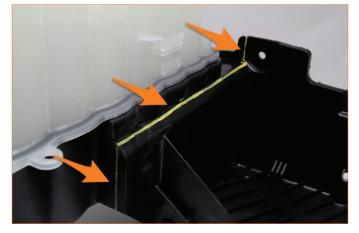
**17.** Using an angle grinder with a cutting disc, cut along the line drawn on the battery tray.
