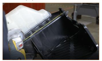
**18.** Using a reciprocating saw, remove the support ribs from the bottom side of the stock degas tank.
