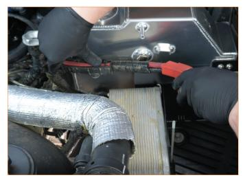
Reinstall the hot-side intercooler pipe. (3x constant-tension T-bolt clamps).
