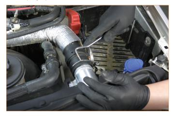
06. Remove the hot-side intercooler pipe from the vehicle. (3x constant-tension T-bolt clamps).
