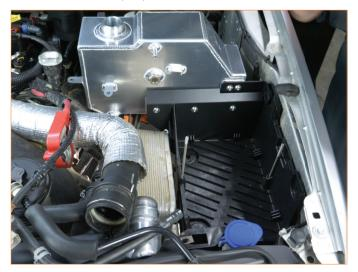
Adjust the degas tank so that it is level and then tighten the 5x allen bolts. (5x 5mm allen bolts).
