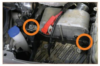
14. Remove the bolts securing the battery tray to the vehicle. Once the bolts are removed, lift the battery tray/primary degas tank out of the vehicle. (4x 13mm bolts).
