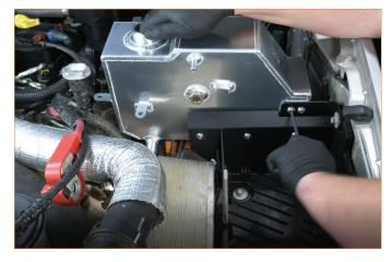
Reinstall the intercooler to the side of the battery tray. (2x 13mm bolts).
