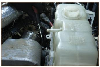
Remove the bolts securing the intercooler to the battery tray. Once the bolts are removed, lift the intercooler to unseat it from the battery tray, then push it towards the engine and set it back down. (2x 13mm bolts).
