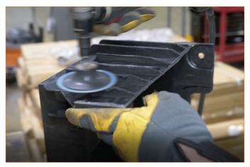
21. Place the MM2356-03 bracket into the battery tray as shown in the image below and mark the 3 holes. Using a 3/8" drill bit, drill the 3 holes in the battery tray.
