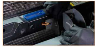
07. Remove the bolt that secures the horn assembly to the radiator support. Then lay the horn assembly over the intercooler. (1x 10mm bolt)
