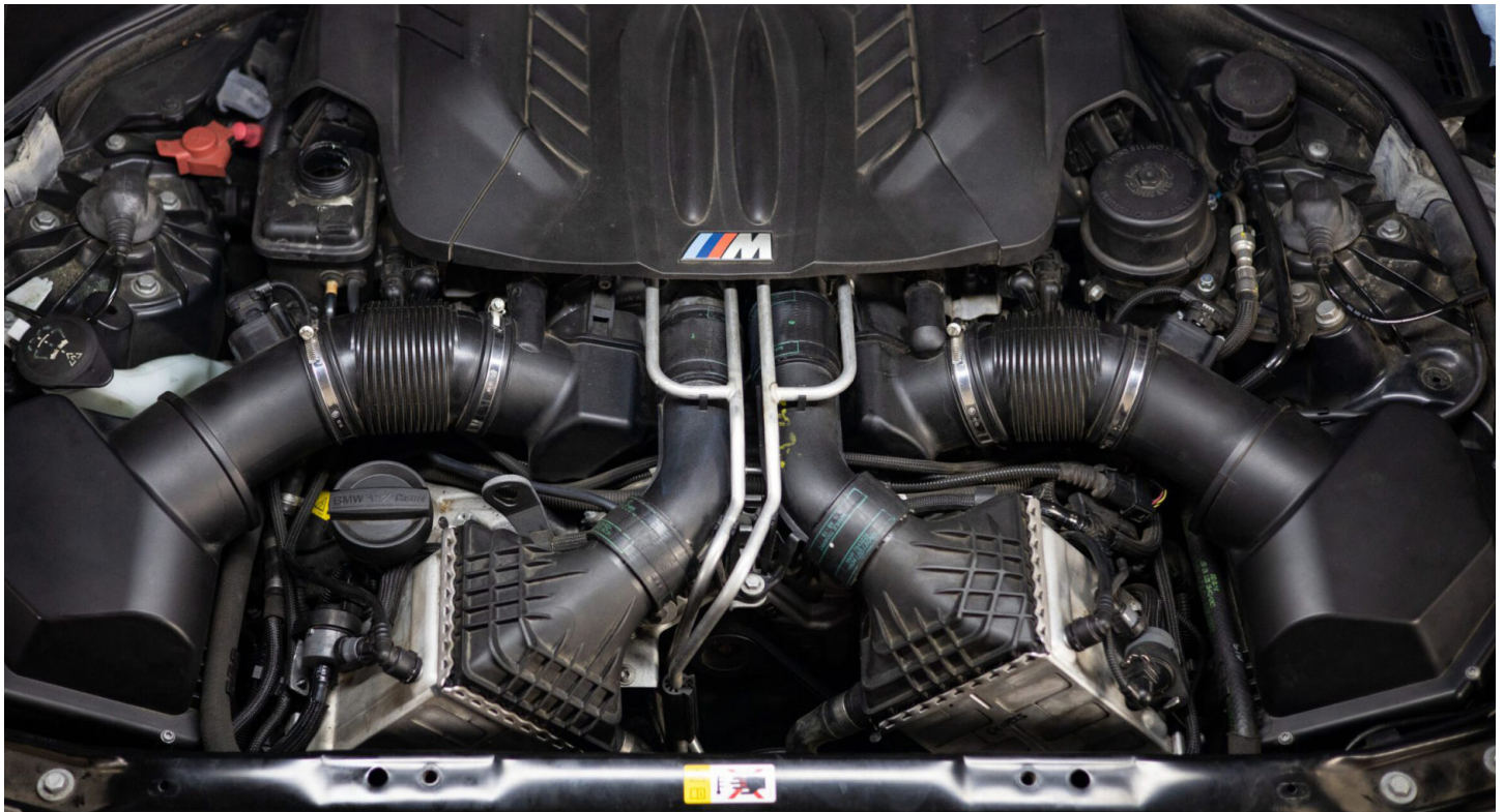
Figure 1: S63 engine employs dual air-to-water intercoolers that move the charge air from the turbo outlets to the intake manifolds located on the sides of the engine.
