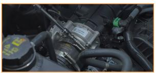
12. Disconnect the air temperature sensor on the cold-side pipe. Depress the tab at the center to separate the connection.
