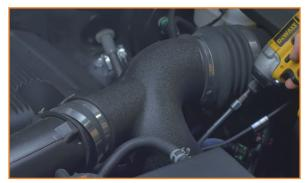
3. Disconnect the air temperature sensor on the intake.
