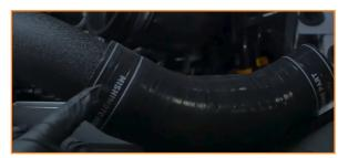
26. Feed the pipe past the front of the engine down to the intercooler. The end without the coupler goes down first and connects to the lower coupler on the intercooler.
