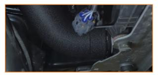
31. Add the 90° section of the cold-side piping to the end of the section already installed to the intercooler. (1x 70-92 worm gear clamp)
