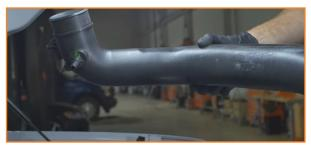
18. Lift the two upper portions of the hot-side piping out of the engine bay. This pipe will also need to be adjusted as you pull it from the engine bay.
