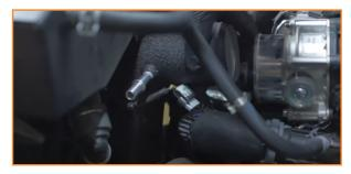
32. Connect the cold-side pipe to the throttle body using the small coupler.(2x 70-92 worm gear clamps)
