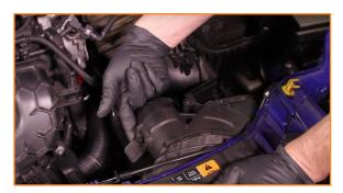
15. Remove the bolt that secures the front section of the intake pipe to the valve cover. (1x 8mm bolt)
