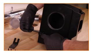
2. Locate the short bracket in your kit and secure it to the Mishimoto airbox with two supplied Allen bolts. (2x 2.5mm Allen bolts)
