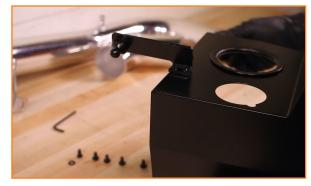
4. Locate the slotted hole in the bottom of the airbox. Secure the second mounting peg to this
