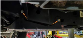
\*If an OEM splash guard is equipped (instead of a skid plate) remove the (2) bolts that attach the (2) brackets to the frame as well as the clip nuts. There is (1) on the driver side and (1) on the passenger side. These bolts, clip nuts, and brackets will not be reused. (4) supplied clip nuts will need to be installed at these mounting locations.
