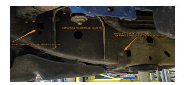
**04.** Using a 13mm socket, install the Borne Off-Road transmission skid plate by reinstalling the (4) bolts removed in step 3 (the (4) supplied bolts, flat washers, & lock washers if an OEM splash guard was equipped) and tighten to 22 lb-ft (30 N-m).
