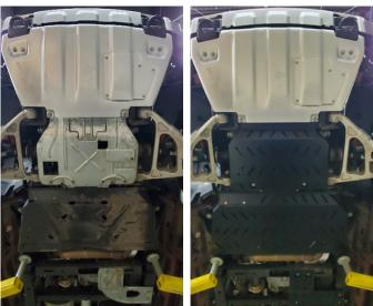
Note: The engine, transmission, and transfer case skid plates are shown above. These installation instructions are for the engine skid plate only.
