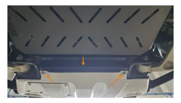
**06**. Using a 13mm socket, install the (2) bolts removed in step 4 and tighten to 22 lb-ft (30 N-m).
