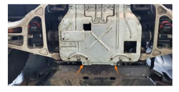
**04.** Using a 13mm socket, remove the last (2) bolts and the engine skid plate from the vehicle.
