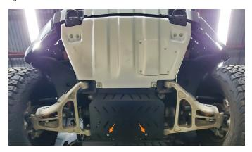
**07.** Using a 10mm socket, install the (2) bolts removed in step 3 and tighten to 106 lb-in (12 N-m).
