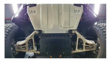
**08.** Using a 13mm socket, tighten the (4) bolts on the front skid plate (if equipped) that were loosened in step one to 22 lb-ft (30 N-m).
