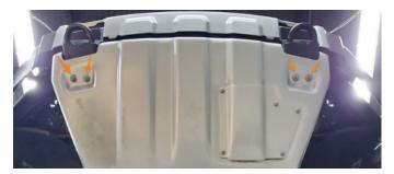
**02.** Using a 15mm socket, remove the (2) rear bolts and the spacer bar (if equipped) between the front skid plate (if equipped) and engine skid plate. Let the front skid plate hang on the (4) bolts that were loosened in step 1.
