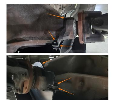
**03.** Tighten the bolts from step 1. Do not overtighten or damage to the axle tube may occur.
