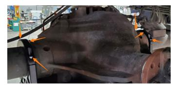
**02.** Using a 6mm allen socket or wrench, install the differential clamp with the supplied (2) 25mm bolts, flat washers, & lock washers. The supplied (2) rubber washers should be placed between the differential clamp and the mount on the skid plate.
