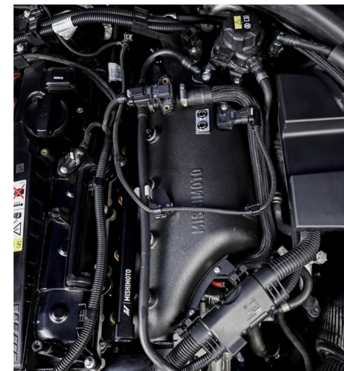
Figure 11: Mishimoto prototype intake manifold installed in a G80 M3. All the brackets and features of the factory manifold are incorporated for an easy installation and great fit and finish.
