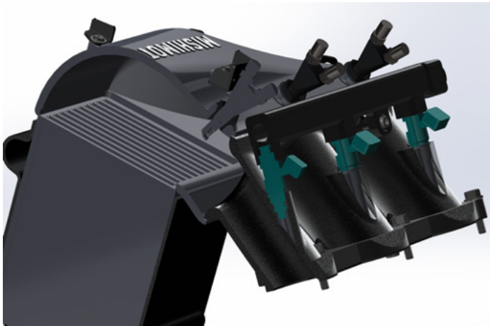
Figure 16: This cutaway shows the optional port injection and nitrous injection features of the Mishimoto Manifold.
