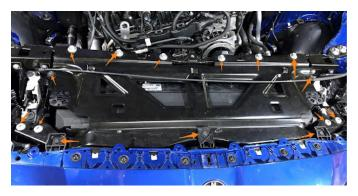
**13.** Remove the 4x pop clips behind the bumper that hold the radiator shroud to the radiator support panel. These clips may require you to pull back on the bumper for better access to the pop clips. Remove the radiator support panel from the vehicle.
