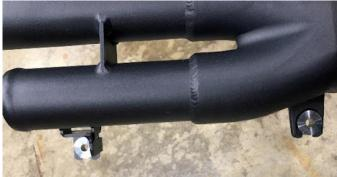
**30.** From underneath the vehicle, remove the spacer for the lower right side Y-pipe attachment point with a 17mm wrench or socket and replace with the included longer spacer. Torque to approx. 8 lb-ft.
