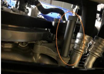
**31.** Install the included throttle body adapter onto the throttle body with the factory bolts. Torque bolts to approx. 8 N-m (6 lb-ft). The adapter should only be able to be installed in the correct orientation.
