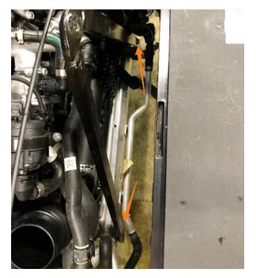
**19.** Locate the auxiliary water pump next to the alternator and remove the 1x 10mm nut. Lift up on the water pump to free it from its mount. This will make it easier to access the sensors in the charge pipe.
