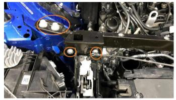
**15.** Remove the upper radiator pipe from both the engine and the radiator, as well as the two smaller hoses attached to it. In addition, remove the small overflow line going from the radiator to the coolant reservoir.
