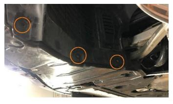
04. Remove the 10mm screws securing the rear undertrays to the vehicle. (Images on next page)
