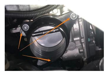
**26.** With a 17mm 12-point socket or wrench, remove the air temp sensor from the factory Y-pipe. Remove the T20 screw from the MAP sensor and remove the MAP sensor from the Y-pipe.
