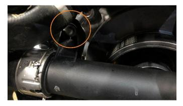
21. Locate the MAP sensor and temperature sensor in the outlet of the Y-pipe, next to the A/C compressor. Disconnect both electrical connectors. Moving the auxiliary water pump out of the way will help give access to the connectors. Both connectors have a white locking tab that must be pulled back to remove the connector.
