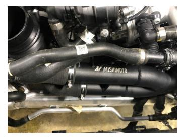
**39.** Reconnect and lock the electrical connectors for the intake temperature sensor and MAP sensor on the outlet of the Y-pipe.
