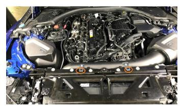
**11.** Remove the front hood seal by pulling up on the seal. Remove the 6x pop clips securing the front plastic panel to the vehicle and remove.
