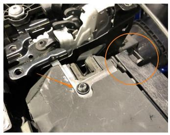
**18.** Remove the 2x 16mm bolts from the lower V-Brace and remove from the vehicle. There will be a coolant hose clipped to the driver's side of the brace. Remove the hose from the clip before removing brace from the vehicle.
