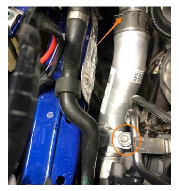
**24.** Remove the quick-connect clamp from the elbow connected to the throttle body and remove the elbow from the vehicle.
