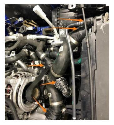
**16.** Remove the lower radiator hose from the radiator and the fan shroud electrical harness. Place the electrical harness to the side.
