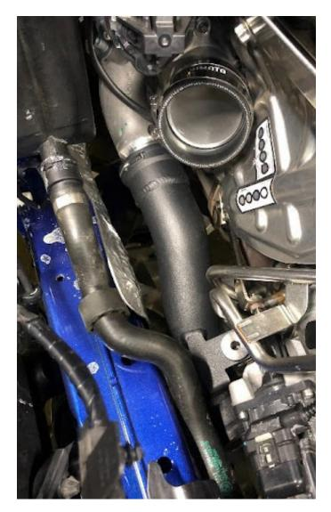
**35.** Install the front turbo boot onto the front turbo adapter. The slightly smaller end will go onto the front turbo adapter and the slightly larger end will go onto the lower inlet of the Y-pipe. Install the rear turbo boot onto the rear turbo pipe. The shorter end will go onto the rear turbo pipe and the longer end will go onto the Y-pipe. Refer to the parts diagram for further details. Install 2x 40-64mm worm gear clamps onto each boot, but do not tighten.
