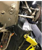
**05.** In each wheel well, remove the 2x (4x total) 10mm screws securing the large aluminum undertray to the wheel well liners.
