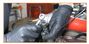
8. Remove the bolts and brackets that secure the radiator. (4x 10mm bolts)
