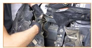
Separate the horn, power steering cooler, and hood latch that are attached to the front of the support bar. (5x 10mm bolts)
