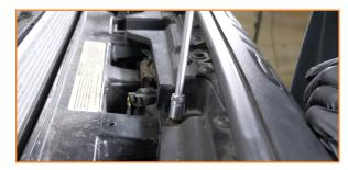
Remove the clips on the grille on both the driver and passenger side. (2x pop-clips)
