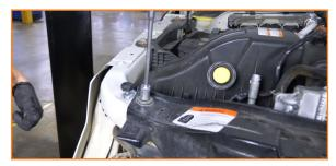
7. Separate the electrical connector from the support bar and remove the hood sensor bracket. (1x 10mm Bolt)
