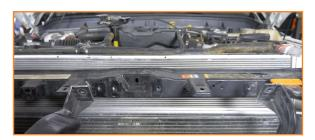
6. Remove the bolts that secure the upper support bar to the front end. (6x 13mm bolts)
