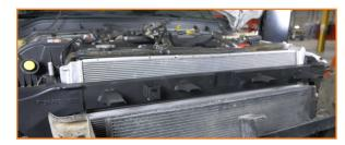
11. Secure the radiator using the radiator support brackets from your kit.
