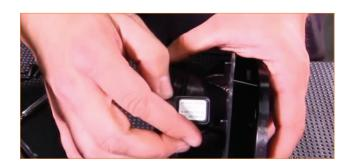
19. Install the stock airbox mounting bracket onto the Mishimoto airbox. Orient the bracket so the dowels point downward, in the same direction as the dowel on the airbox. The 7mm bolts install from inside the box, through the smaller holes. The 10mm bolts install from outside the box, through the larger holes. Orient the bracket so it is flush with the side of the box before fully tightening the bolts. (2x 7mm nuts and bolts, 2x 10mm nuts and bolts)
