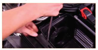
08. Separate the wiring harness connector on the side of the airbox. Push the gray tab out of the connector and then depress the tab to release the connector.
