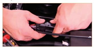
09. Remove the female end of this connector from the airbox. To release the connector, slide a small screwdriver between the connector and the airbox to depress the locking tab. Then slide the connector down and off the airbox.
