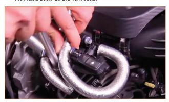
13. Remove the bracket that held the PCV/boost solenoid assembly you just removed. Remove the bolt that secures it, and then wiggle the bracket to aid in removal. (1x T45 Torx bolt)
