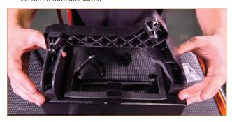
20. Install the ECU onto the airbox. Position the ECU so the cooling fins are inside the airbox and the posts on the ECU fit inside the holes of the airbox. Then install the provided bracket and secure it with two 10mm bolts. (2x 10mm bolts)
