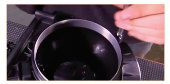
18. Release the MAP sensor from the adapter by turning it counterclockwise, and then remove the sensor.
