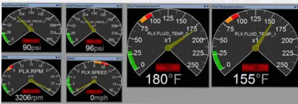
**Figure 1: PLX sensor modules were used to monitor engine pyrometers.**
