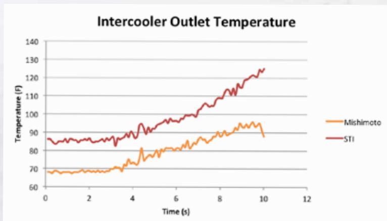
**Figure 3: The Mishimoto intercooler outlet temperature shows an average decrease of 15 °F and a maximum of 30 °F.**
