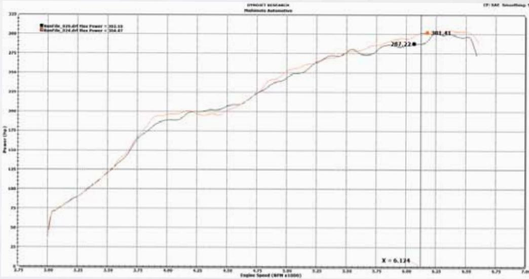
Figure 6: Mishimoto intercooler shows gains of up to 14 hp in the 5500+ rpm range.
