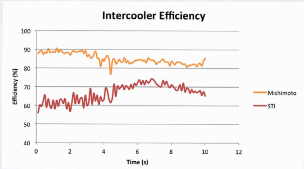
Figure 4: The Mishimoto intercooler shows an average efficiency of about 85% compared to the STI efficiency of approximately 70%.
