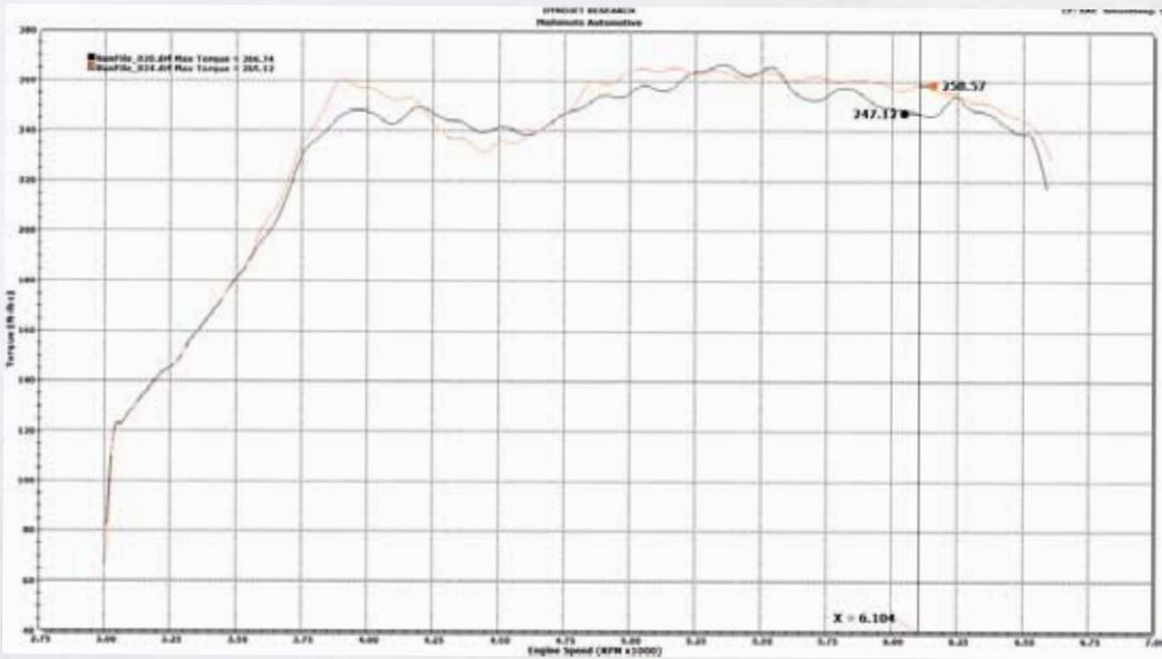
Figure 7: Mishimoto shows significant torque gains of up to 11 ft-lb in the 5500+ rpm range.
