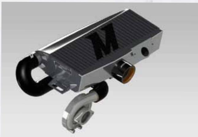
**Figure 2: CAD rendering of the intercooler before first prototype**
