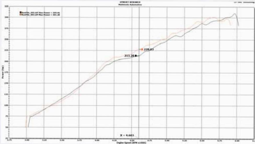
Figure 8: Mishimoto intercooler shows improved power across the entire power band, with a maximum gain of 15 hp.
