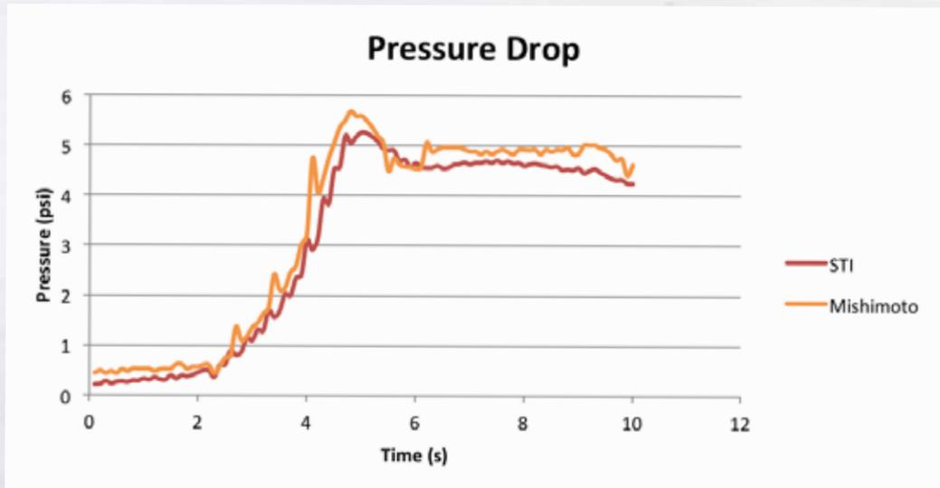
Figure 5: Mishimoto intercooler shows little increase in pressure drop compared to the STI.
