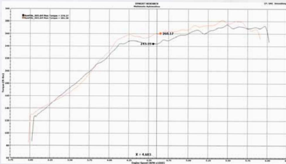
Figure 9: Mishimoto intercooler shows torque gains across the entire power band, with a maximum gain of 17 ft-lb
