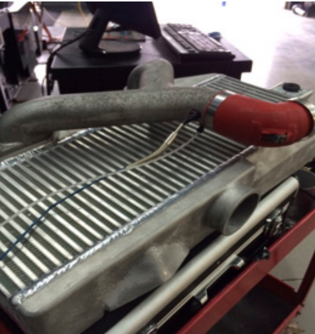
FIGURE 2: Mounting locations for temperature and pressure sensors, which read approximately 10 times per second.
