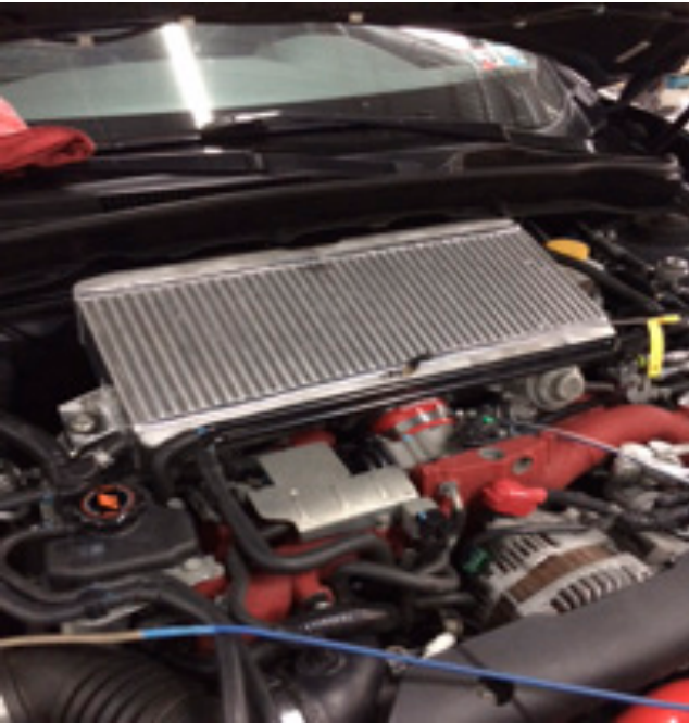
FIGURE 3: Mounting locations for temperature and pressure sensors, which read approximately 10 times per second
