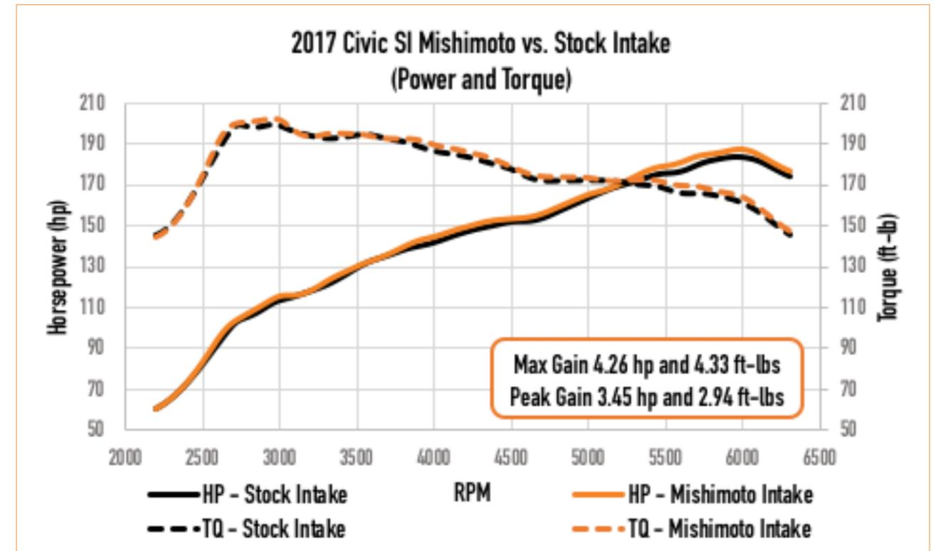
FIGURE 4: Dyno result (power and torque).
