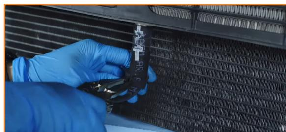
14. Remove the bolts on the transmission cooler bracket. (2x 10mm bolts)
