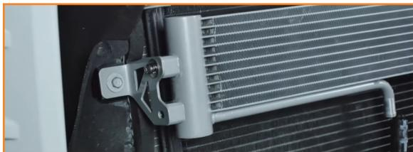
17. Adjust the transmission cooler so that it is parallel with the condenser. Then fully tighten all hardware.
