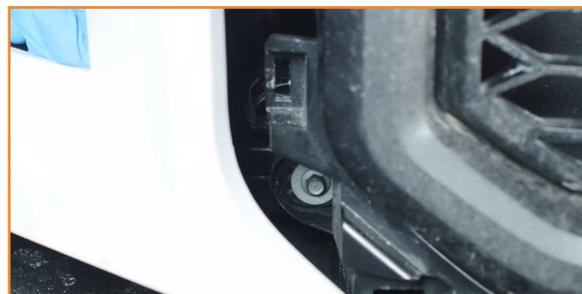
10. Release the clips on each side of the grille. You will need to lift the grille to reach these clips. (2x tree clips)
