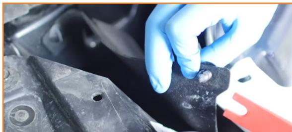
6. Disconnect the grille shutter, camera, and washer fluid harnesses. These can be found in front of the hood latch connector.
