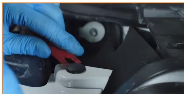
3. Release the clips that secure the radiator cover and remove it. (8x pop-clips)
