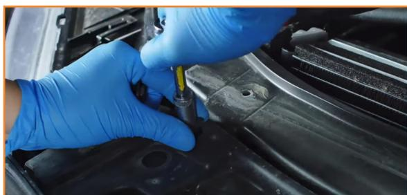
9. Remove the bolts at the bottom of the grille. These are located at the back of the grille and will be difficult to reach. (2x 8mm bolts)
