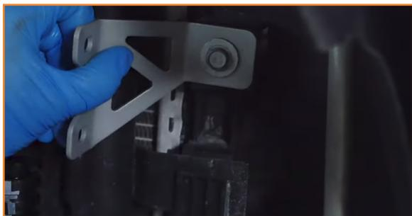
16. Install the transmission cooler to the brackets. The transmission cooler can be installed in two orientations. For the F-150 2.7L & 3.5L EcoBoost, install the cooler with the inlet & outlet facing up, and relocate the tree clip on the hose to the riveted bracket on the bottom. (4x 4mm Allen bolts, 8x washers)
