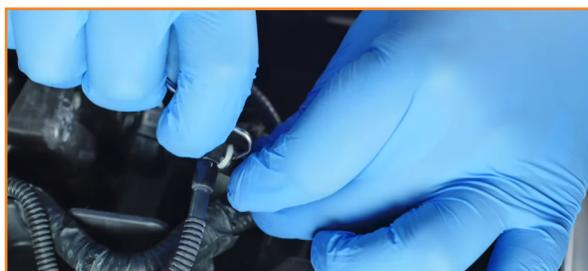
7. Separate the wiring harness from the grille. (2x tree clips)
