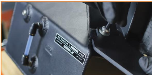
18. Reinstall the battery box with the expansion tank. (4x 13mm bolts)
