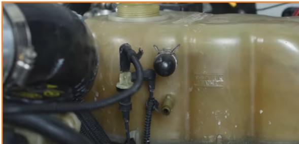
6. Disconnect the return hose from the bottom of the reservoir tank. (1x spring clip)
