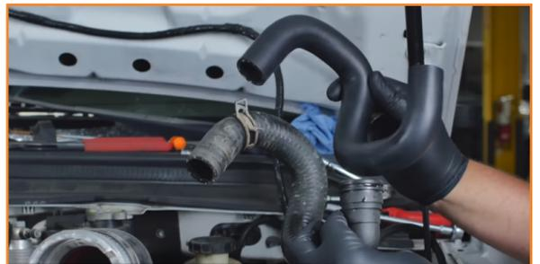
11. Install the Mishimoto hose to the side of the engine. (1x worm gear clamp)
