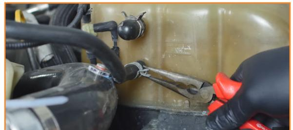
4. Pull out the clip that secures the upper radiator hose to the radiator. Slide the upper radiator hose off the radiator. You need to move the hose out of the way so you can successfully lift the battery tray. (1x spring clip)
