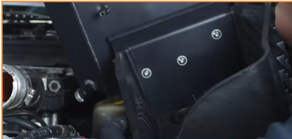
17. Install the included bracket to the expansion tank. (2x 5mm Allen bolts)
