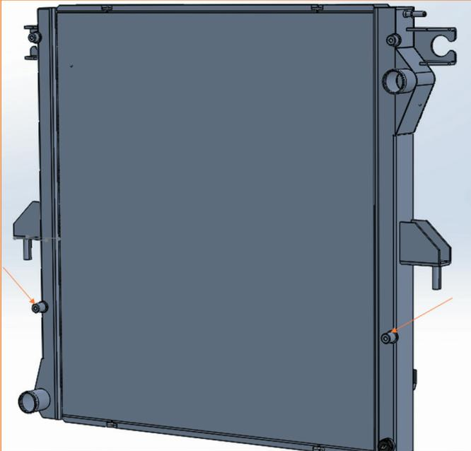
11. Using the provided 2x M4x0.7 14MM long bolts, attach the upper fan shroud to the radiator.
