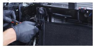
15. Remove the plastic bracket that was formerly securing the AC condenser on the driver side. (2x 13mm bolts, 2x 10mm bolts, 1x pop-clip)
