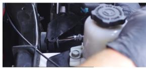
21. Two bolts hold the transmission cooler in place.Remove these bolts, along with the mounting bolt connecting the cooler to the radiator.(3x 10mm bolts)
