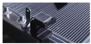
30. Lower the Mishimoto Radiator into the engine bay. Watch for the AC lines and be sure to engage the rubber isolator bushings on the bottom with the crash bar. For older models, connect the
