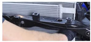
23. Pull the rubber bushings off the radiator brackets.
