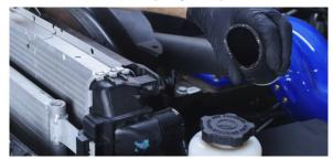
18. Loosen the clamps securing both ends of the hot-side intercooler pipe. Lift the pipe up through the engine bay to remove it.(2x worm gear clamps)
