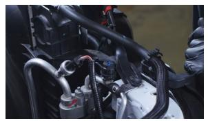
9. Separate the front shrouding on the driver side of the radiator. (3x pop-clips, 1x 10mm bolt)
