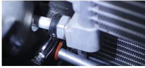
22. Slide the transmission cooler over to get the tabs out from behind the radiator bracket.
