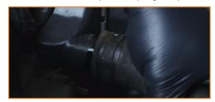
8. Compress the clamp on the lower radiator hose and slide it down the hose. Then pull the lower radiator hose off the port. (1x spring clamp)
