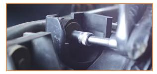
11. Part the transmission cooler from the radiator.Let it rest up against the support beam.(1x 10mm bolts)
