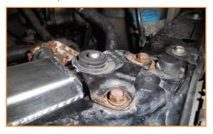
**4.** Plug in the fans and AC compressor. Re-install the lower hose and plug in the fan plugs on lower side of car.
