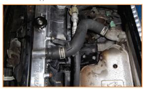
**3.** Re-install the upper mounting points making sure the rubber isolators are in place.
