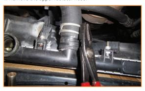
**5.** Remove the brackets from top of radiator to support (10mm head bolts).
