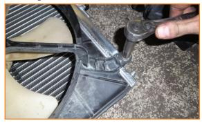
2. Install the Mishimoto radiator into the engine bay making sure the rubber insulators are located in the OEM mounting cups. Re-install the upper coolant hose.
