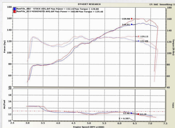
Figure 4: The selected Mishimoto intake provides more horsepower and torque over stock while still closely following the OEM AFR curve.
