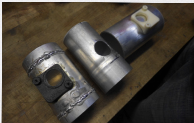
Figure 2: Three pipes of different internal diameters were used for this experiment.
