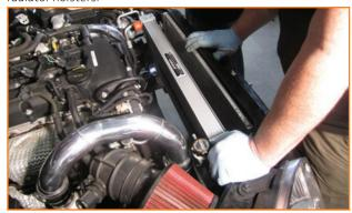
2. Reinstall the (4) 10mm bolts for the radiator stays.
