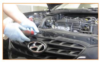
**8.** Locate radiator drain plug and remove fluid from radiator. Drain into an appropriate container.
