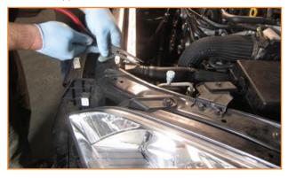
4. Reinstall the (2) 10mm A/C condenser bolts and reinstall the insulator strip.
