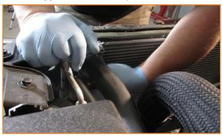
13. Pull off insulator strip on top of the radiator.
