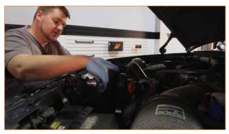
**5.** Reinstall the upper coolant hose to the radiator. Be sure to tighten the clamp.
