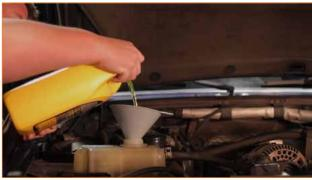
**10.** Start the vehicle and set the heat on high. Allow the vehicle to reach operating temperature so that any air from the cooling system will be purged. Be sure to inspect the cooling system for any leaks.
