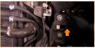
12. Remove the two bolts that secure the transmission cooler to the radiator support. Allow the cooler to droop over the crossover pipe. (2x 10mm bolts)
