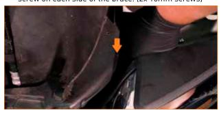
07. Release the tree-clip that secures the bottom of the rubber shroud. Do this on both sides. (2x tree-clips)
