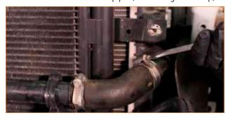
18. Release the two clips from the quick-disconnect fittings on the crossover pipe. Disconnect the upper hose from the crossover pipe by pushing it back, then release the fitting from the thermostat housing by pulling upward. There may be residual coolant inside the system, so keep your bucket handy to capture any spills.
