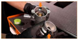
caps with the four provided flange-head bolts. (4x 10mm flange-head bolts)
