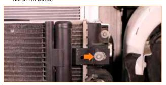
17. Once the coolant has finished draining, loosen the wormgear clamp on the crossover pipe where it connects to the secondary radiator on the driver side, and pull the hose off the radiator. Lift the hose up to allow residual coolant to drain from the crossover pipe. (1x worm-gear clamp)
