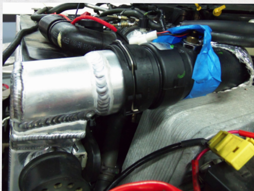
Figure 2: Temperature sensors were placed in the upper and lower radiator hoses before the hose connections.
