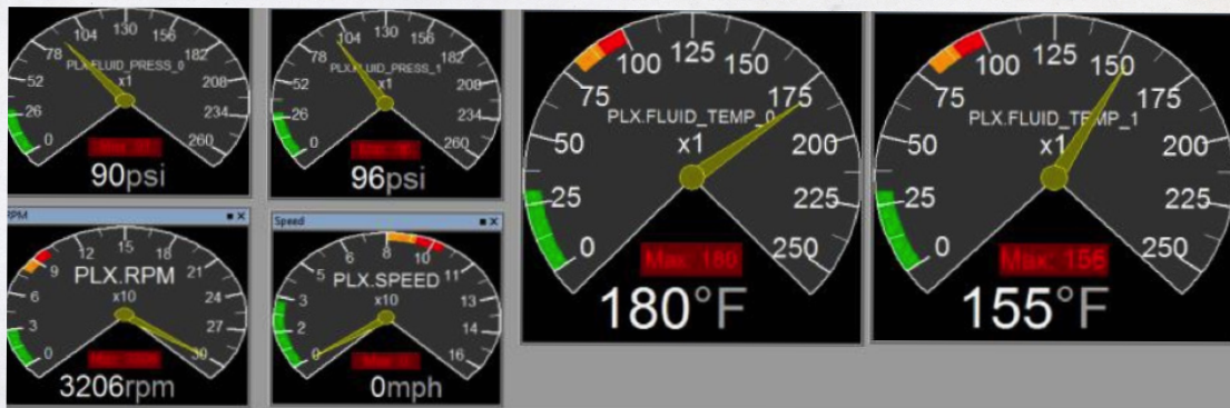
Figure 1: Coolant temperatures were taken at both the inlet and outlet of the radiators using PLX fluid temperature sensors.
