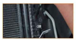
14. Compress the clamp on the overflow hose and reposition the clamp down the hose so it clears the barb. Slide the hose off the radiator port. (1x spring clamp)
