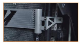
12. Detach the radiator shrouding on each side. Once the bracket is free, move it out of the way and then remove the bolt behind it. (1x 10mm bolt & nut)
