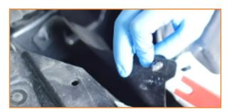
7. Disconnect the grille shutter, camera, and washer fluid harnesses. Separate the wiring from the clips that secure them in place. (2x tree clips)
