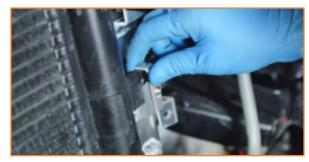
34. Secure the transmission line to the bracket on the radiator using the provided bolt. (1x 10mm short bolt)
