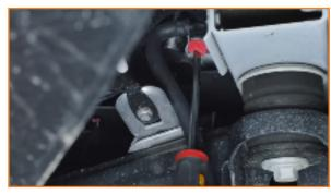
Remove the intake duct. (2x pop-clips, 1x 8mm screw)
