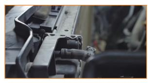
15. Release the shrouding connected to the driver side of the radiator. (2x pop-clips)
