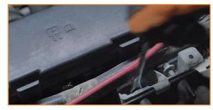
7. Release the clips that secure the nearby wiring to the fan. (2x tree clips)
