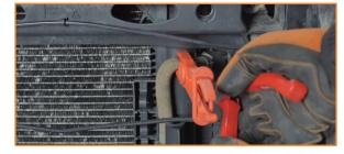
17. Remove the upper and lower transmission lines from the raidator. (2x spring clamps)
