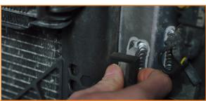
25. Using the two provided brackets, secure the passenger side of the AC condenser. (4x 4mm Allen screws)
