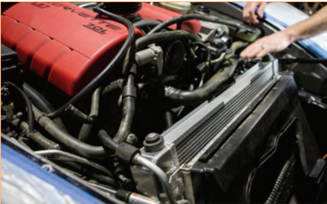
FIGURE 1: The Corvette C6 radiator mounted in the car.
