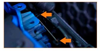
11. Lift the tabs on the radiator support to release the bumper. There is one tab on each side, located underneath the headlight mounting location.
