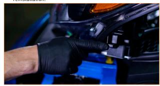
04. Remove the two pop-clips that secure the undertray to the stabilizer bar. (2x pop-clips)
