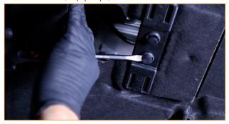
**05.** Remove the eight Torx screws and two pop-clips that secure the undertray to the bottom of the vehicle. Slide the undertray forward, and remove it from the vehicle. (8x T30 Torx screws, 2x pop-clips)
