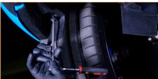
07. Remove the pop-clip and two Torx screws that secure the passenger-side fender liner to the bumper. Then pull back the fender liner to access and remove the pop-clip that secures the bumper to the fender. Pull the upper corner of the bumper away from the fender to release it. Repeat this process on the driver side. (4x pop-clips, 4x T30 Torx screws)
