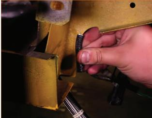
40. Install the oil cooler. Position the oil cooler so that the ports face downward. Align the hole in the left-side mounting bracket with the hole for the inner bolt on the passenger-side headlight. Thread in the original headlight bolt, but do not fully tighten. (1x 10mm bolt)
