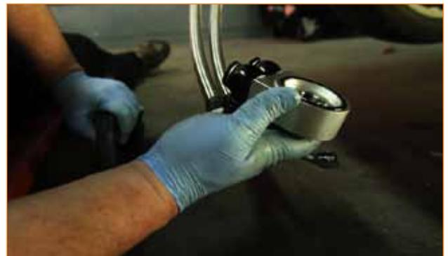
3. Route the lines over the frame towards the location of the oil filter.
