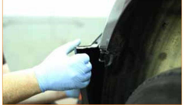
6. Unbolt the horns and attach the horn relocation bracket. The relocated horns should both be on the driver's side of the vehicle.
