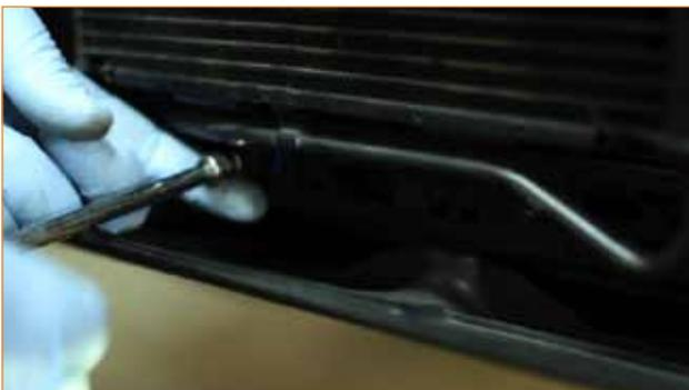
5. Next remove the third bolt located in the front bumper frame, as seen in the photo.
