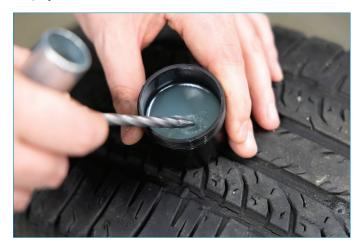
**03.** Push the abrasive reamer tool into the hole slowly, once you feel that you have separated the steel belts within the tire rotate the tool back and forth slowly to make a more uniform sealable hole.
