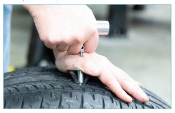
**07.** Once the insertion tool is full removed, use the knife included in the kit to cut any repair cord that is sticking out above the tread.
