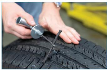
**05.** When you are ready remove the reamer tool from the hole and push the insertion tool and cord into the hole. Do not push so far that the ends of the repair cord go into the tire.
